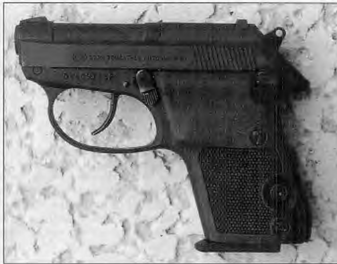
Beretta Tomcat, left-side view — Pearce neoprene-type grip panel was designed to inhibit accidental release of the tip-up barrel.
